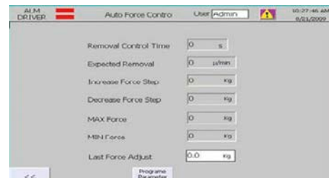
Auto force control Maintains a steady cut rate even for high stock removal rates, enables consistent production removal rates
