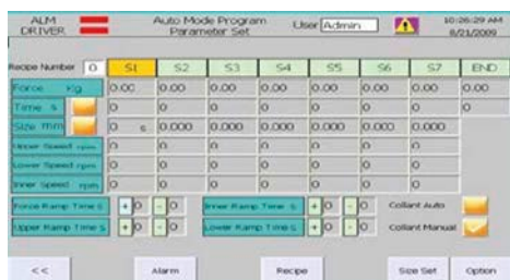
Program storage screen Program storage is available for up to thirty process recipes
