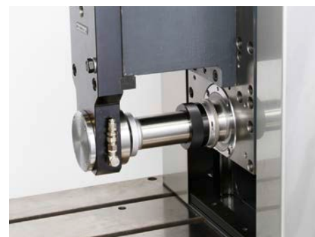
Head mounted diamond roll dressing unit
