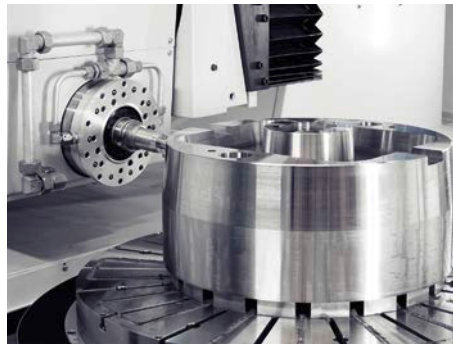
Boring machine processing
