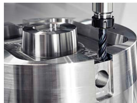
Hard milling (fine machining)
