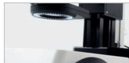
Planapo 1×: the working distance of 61.5mm leaves a lot of free space under the objective
