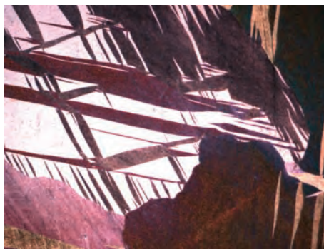
Tin with deformation twins, 1:100
