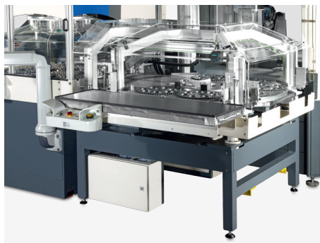
Twin Loader – automatic work piece carrier exchange for shortest loading times
